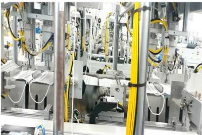
9. Ear-loop welding setting
